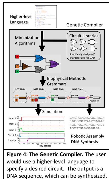
**Figure 4: The Genetic Compiler.** The user would use a higher-level language to specify a desired circuit. The output is a DNA sequence, which can be synthesized.
