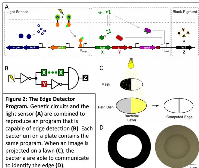
**Figure 2: The Edge Detector Program.** Genetic circuits and the light sensor (A) are combined to reproduce a program that is capable of edge detection (B). Each bacterium on a plate contains the same program. When an image is projected on a lawn (C), the bacteria are able to communicate to identify the edge (D).
